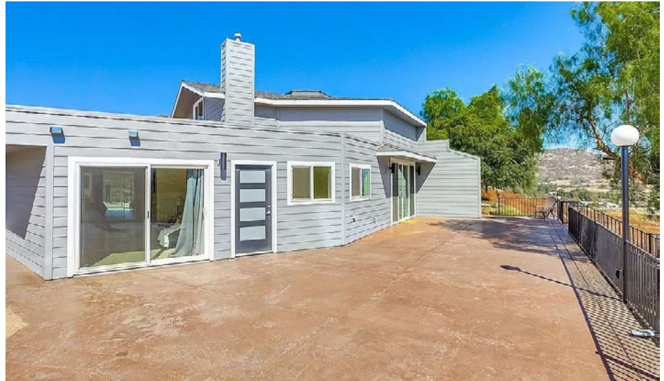
Linda O'Brien has hardened her home to make it less likely to burn in a wildfire, including adding fire-resistant features such as a non-combustible patio, rock landscaping around the property, an asphalt roof and Hardie board siding—with no vegetation in Zone 0.
